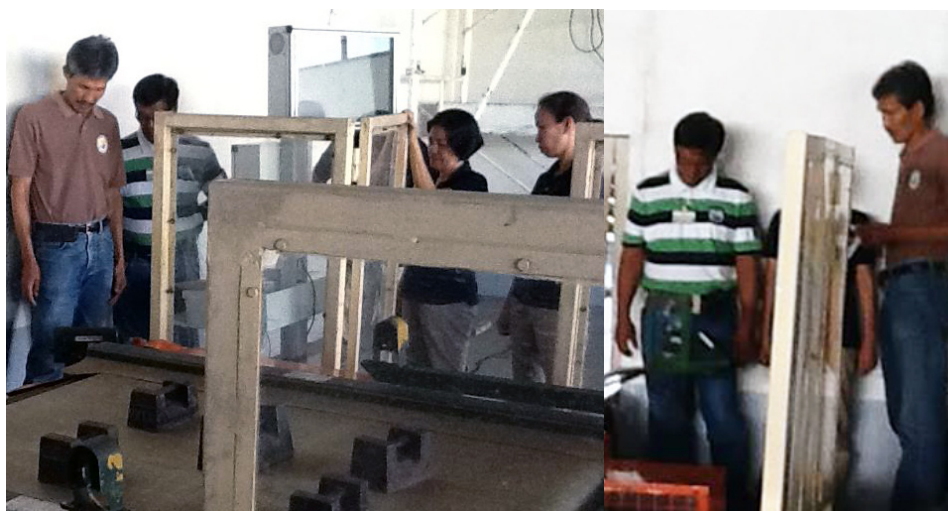
CALIBRATION/SEALING OF WEIGHING SCALES. Faustino O. Taal, OIC NTA Vigan Branch, and Senior TPRO Gilbert I. Yadao, placed calibrated weights onto a weighing scale in a trading center in Vigan to ensure the accuracy of weighing and measuring instruments in preparation for the tobacco trading season in the first district of Ilocos Sur. The Vigan branch conducted early February the calibration and sealing of weighing scales in four trading centers in Cabugao, Ilocos Sur and one in Vigan City. NTA Vigan
